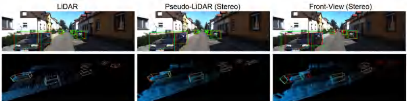
图表60: Pseudo-LiDAR 点云生与激光雷达、前向视觉对物体感知的识别对比
